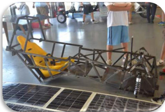
Completed Frame in the Garage at the TMS
